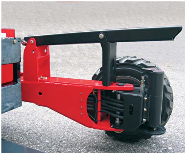
Precise hose routing guarantees longest service life
