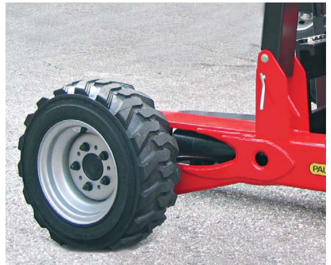
Retracted steering cylinders = optimal protection during transportation on the truck
